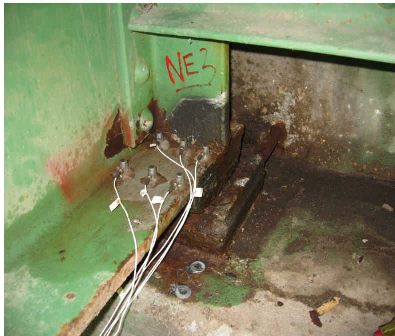
Figure 4.45 Forced vibration response measurement of northeast end and boundary condition of beam 3
