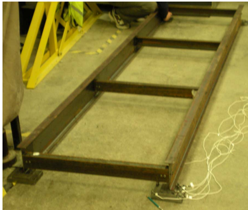
Figure 3.21 Scale bridge in the laboratory
