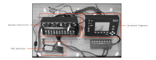
Figure 38: Mobile System Laboratory Configuration
