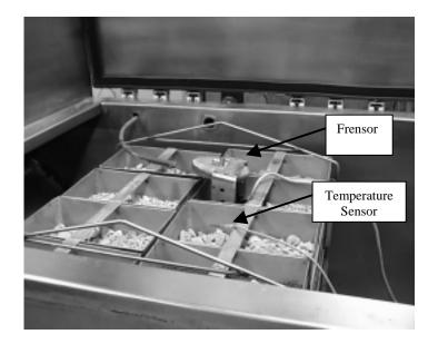
Figure 26: Frensor sensor placed in freezer
