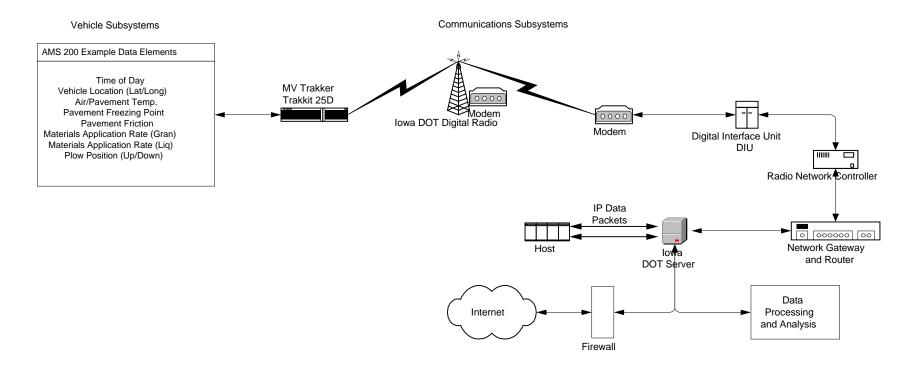
Draft-CTRE DKroeger Work in Progress Phase IV Concept Vehicle Communications System Diagram DRAFT 10/22/2001
