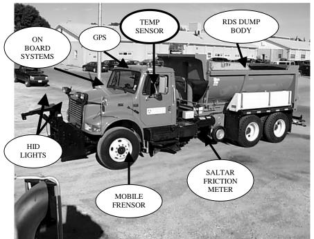
Figure 3: Phase IV Highway Maintenance Concept Vehicle
