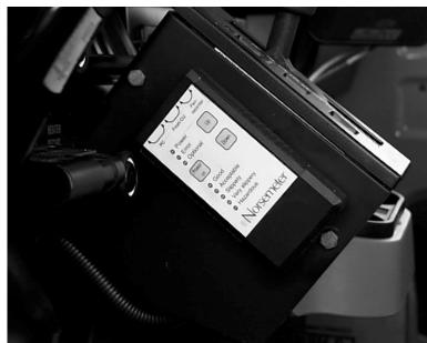
**Figure 13: Operator Panel Installed in Truck**
