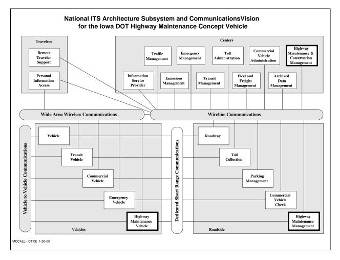
Figure 5: National ITS Architecture with HMCV Vision
