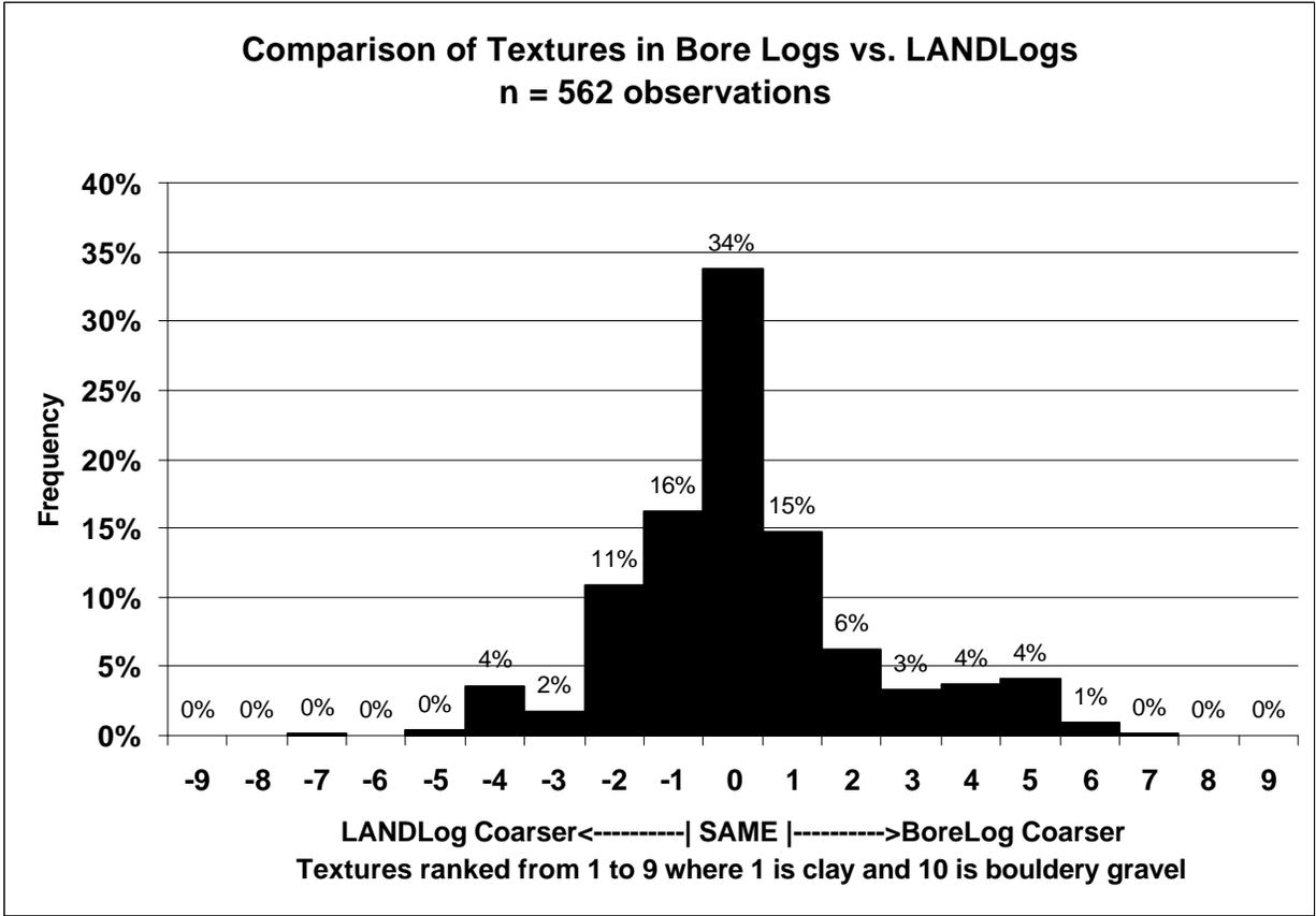
Figure 8. Graphic comparison of sediment textures in geotechnical vs. archaeological logs
