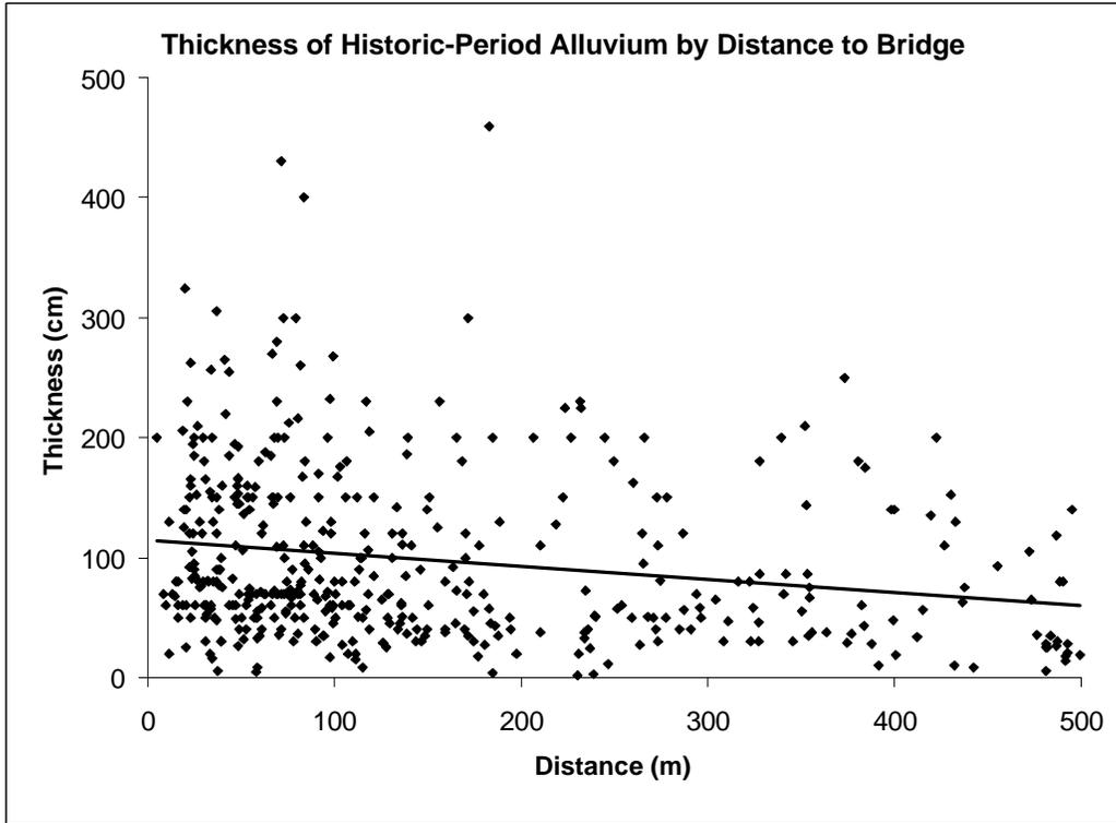
Figure 16 Historic alluvium thickness plotted against distance to bridge.
