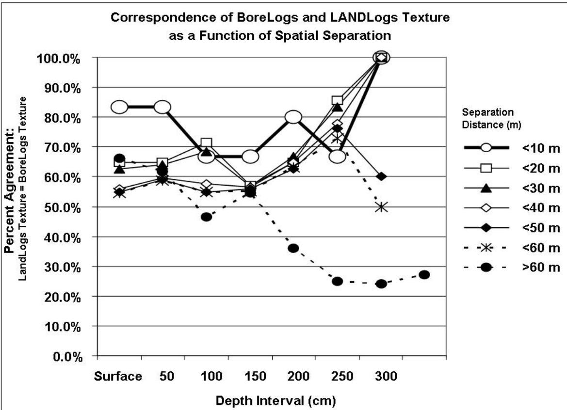
Figure 9. Agreement between sediment textures in geotechnical vs. archaeological logs as a function of hole proximity and depth interval.
