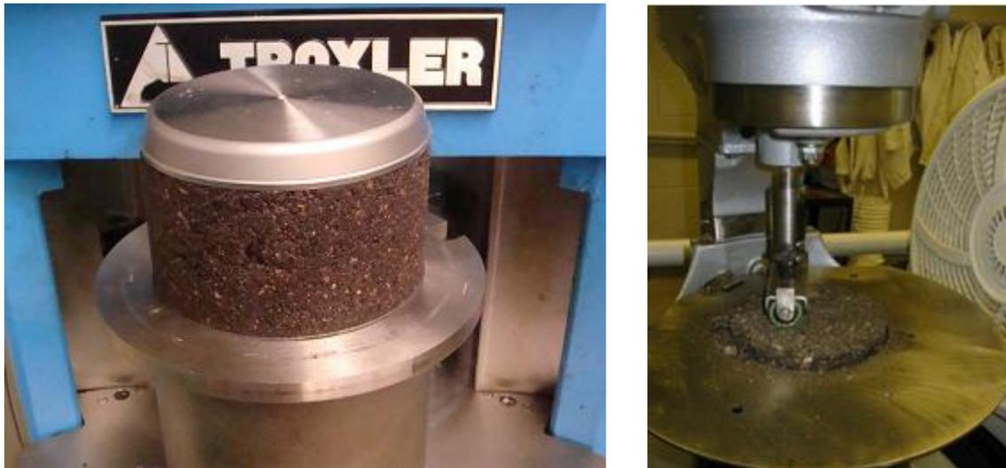
**Figure 8-22. Pictures of raveling testing specimens and equipment**
