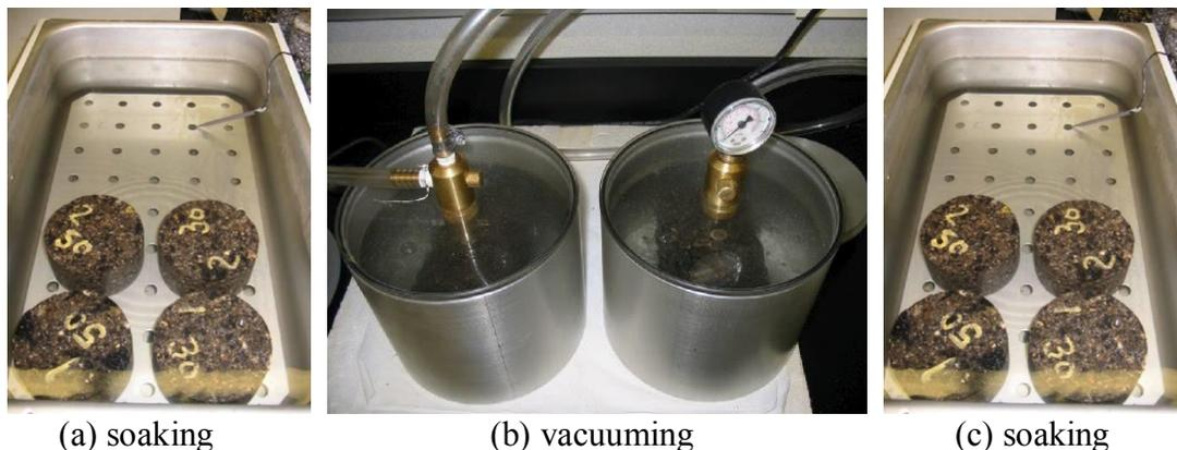
**Figure 7-10. Vacuum saturation procedure for making wet specimens**
