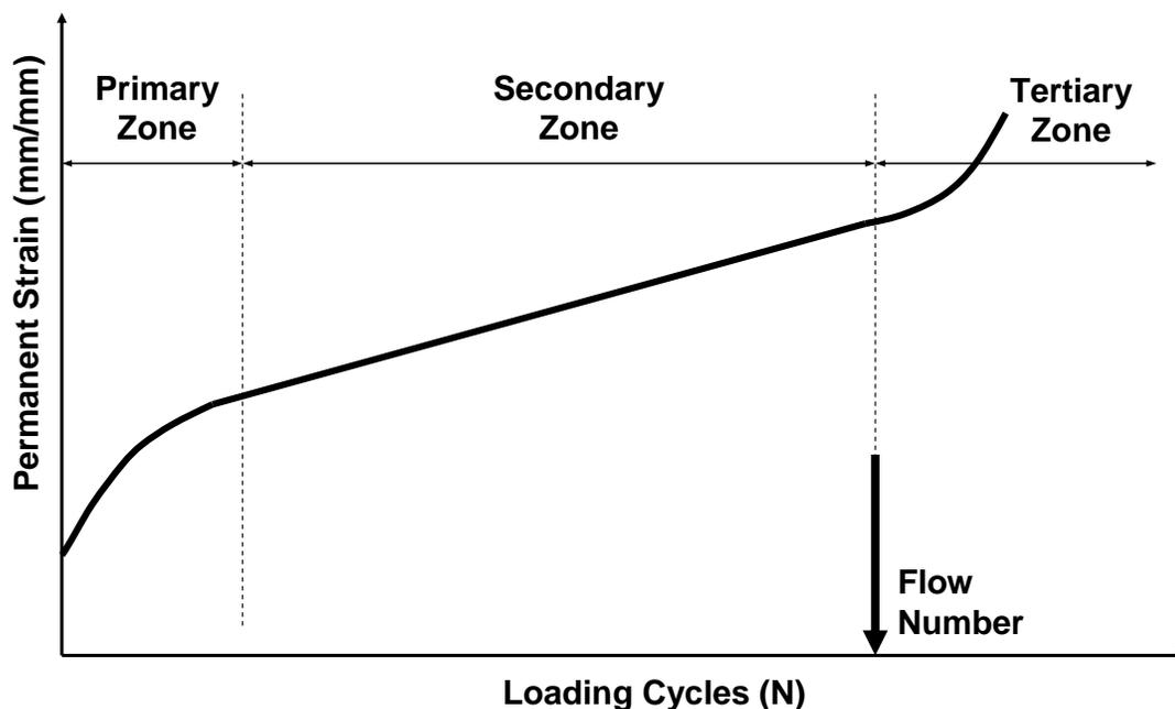
Figure 8-11. Permanent deformation behavior against loading cycles
