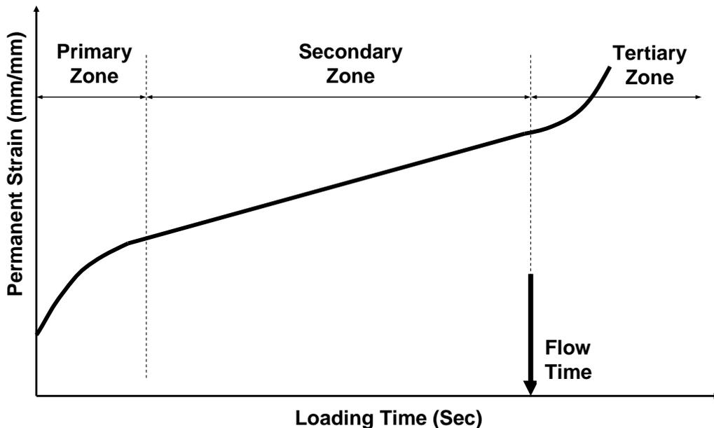
Figure 8-15. Permanent deformation behavior against loading time
