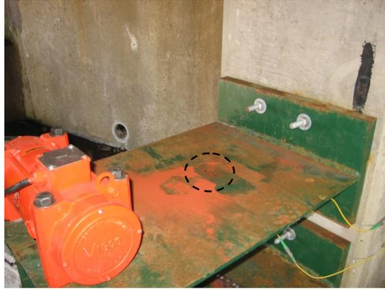
a. Overview of Top Web-Plate Cracking
