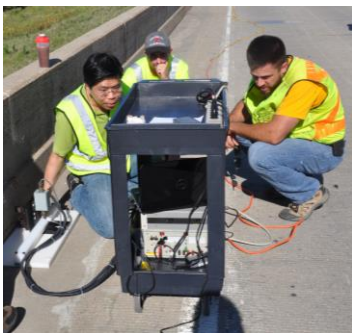
Figure 37. Iowa Highway 210 Bridge MFL field testing
