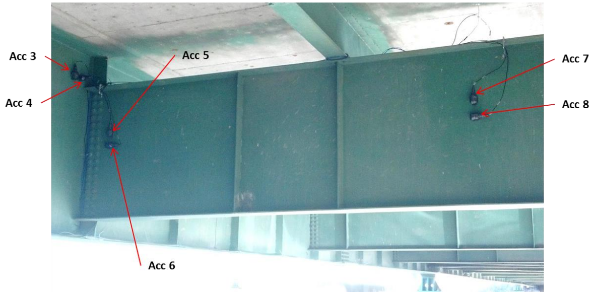
Figure 14. Sensor orientation for Section A
