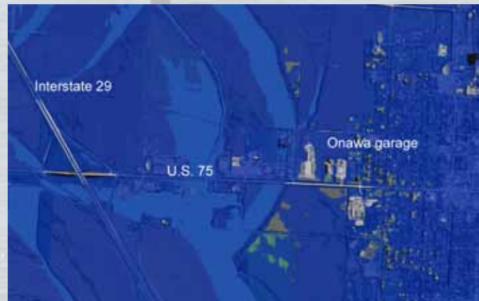
LiDAR was used to show the worst case flood elevation in Onawa to assess the flood risk to the Iowa DOT's garage. This assessment showed that even in the worst case, the garage would not be included. This saved significant resources as the stored salt and sand would not have to be moved.
