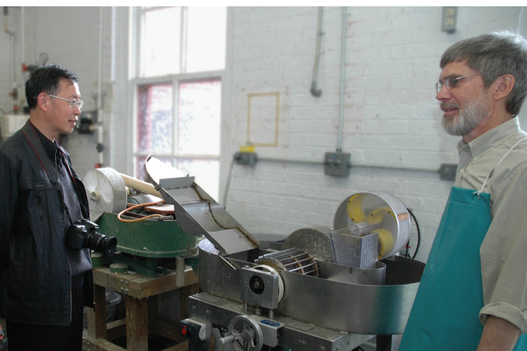
Tim Barrett (right) explains the operation of the hollander beater used to prepare pulp from cellulose fiber.
