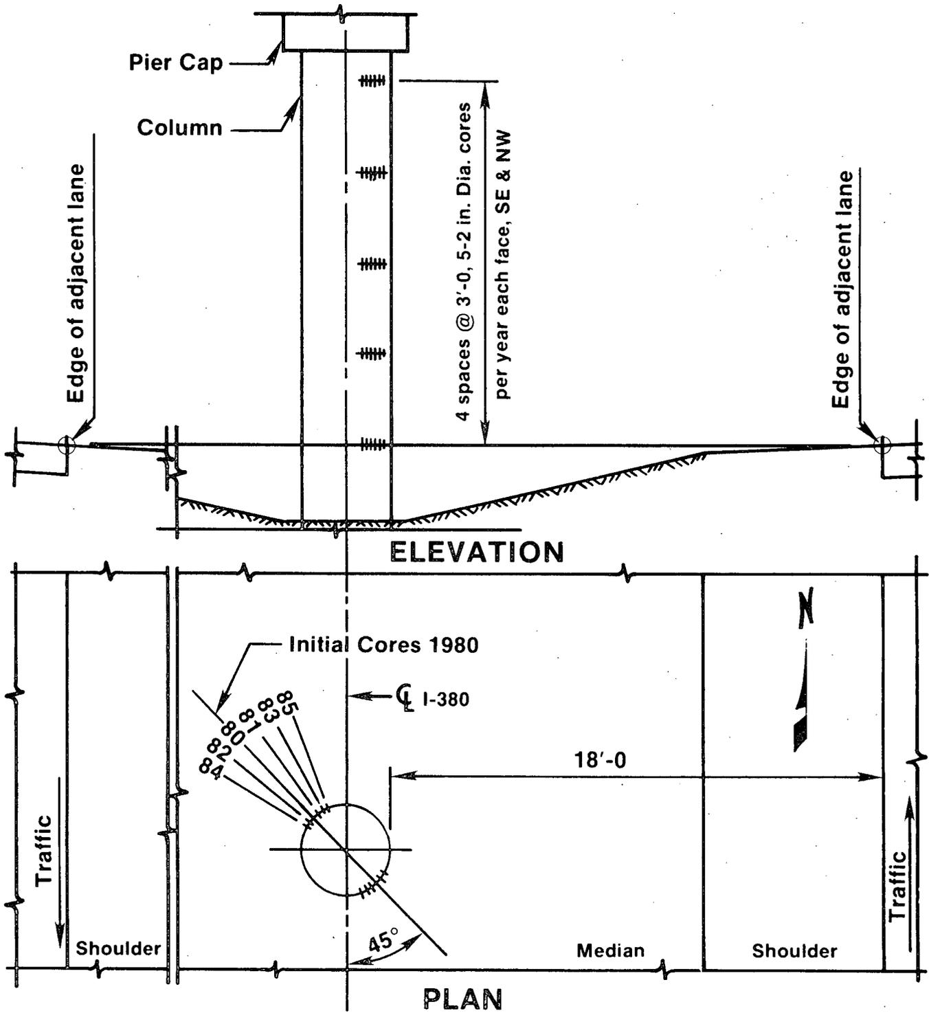
**FIGURE 3 - I-380 CORE SAMPLING PLAN**
