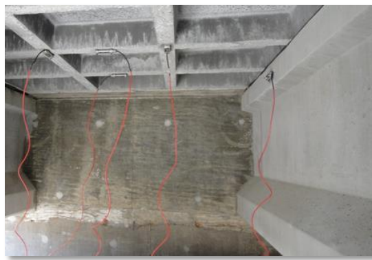
Figure 4.5. Transducers under deck adjacent to abutment face
