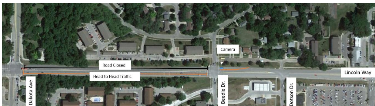
Figure 10. Lincoln Way work-zone layout
