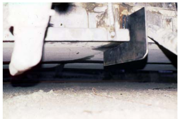
Figure 3. Front mounted joint forming knife, near paver vibrators.
