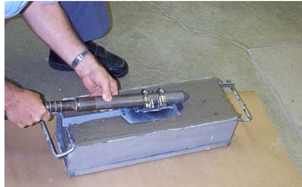
Figure 1. Laboratory vibrator and beam mold with concrete for initial joint forming test.
