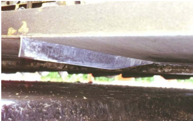
Figure 4. One of the twin parallel rear mounted joint forming knives.
