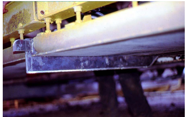
Figure 2. Rear mounted joint forming knife under the floating pan.
