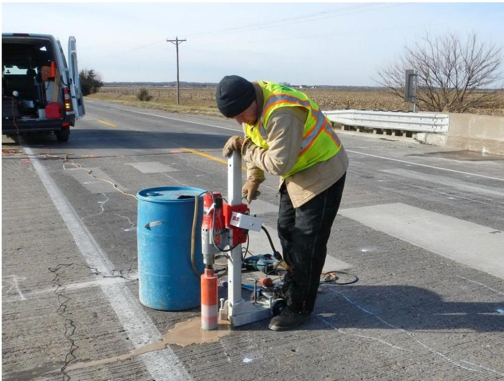
*Figure 2.2. Drilling a core sample from the deck.*
