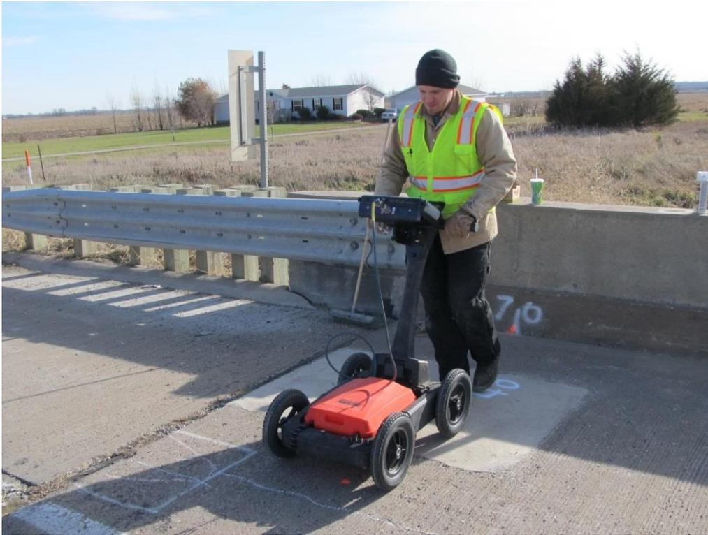
*Figure 2.1. Measuring reinforcing cover depth with GPR.*
