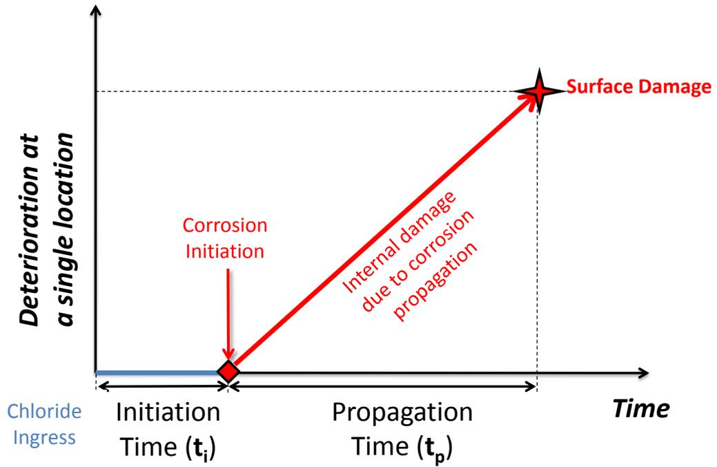
Figure 4.1. Corrosion sequence (adapted from Tuutti 1982).
