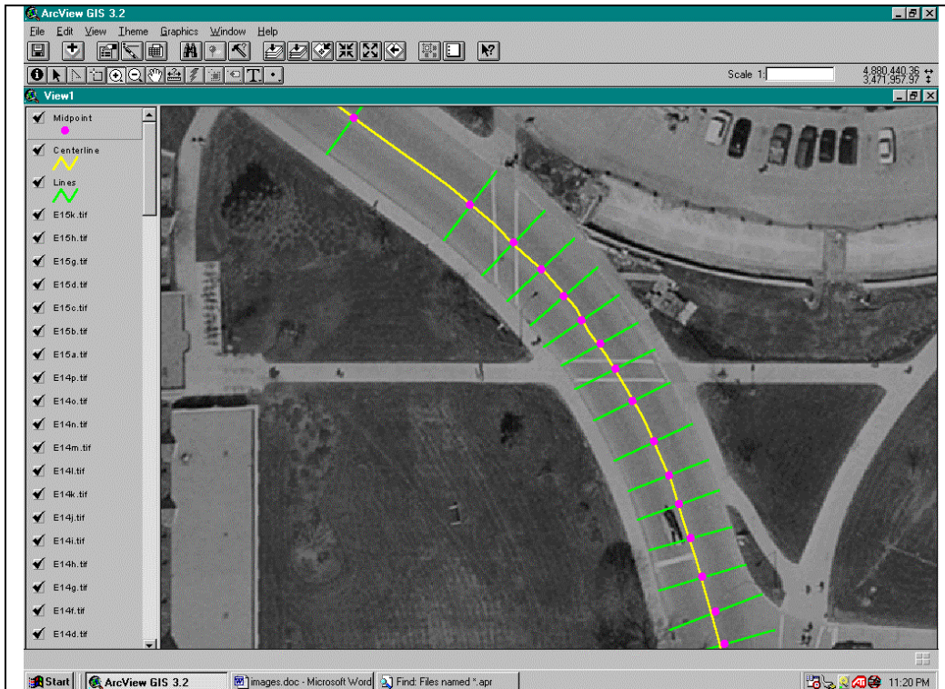
Figure 5-3: Calculation of Roadway Centerline
