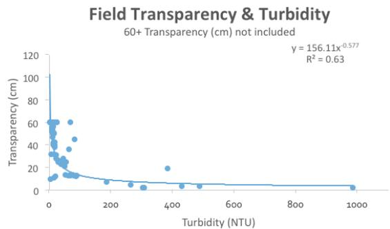
Figure 48 – Relationship between the lab transparency and turbidity measurements
