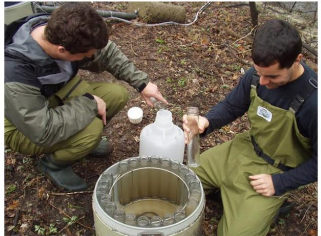
Figure 42: Teledyne ISCO automated sampler with composite water samples following a triggered storm event. With a high degree of accuracy and precision, use of ISCO samplers also come at a high price and a high degree of required calibration.
