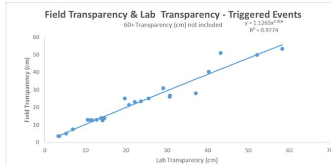
Fig. 54 : Field Transparency vs Lab Transparency for Triggered events - 60 cm excluded.  $r^2 = .9774$
