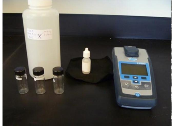
Figure 38 – Hach 2100Q turbidimeter
