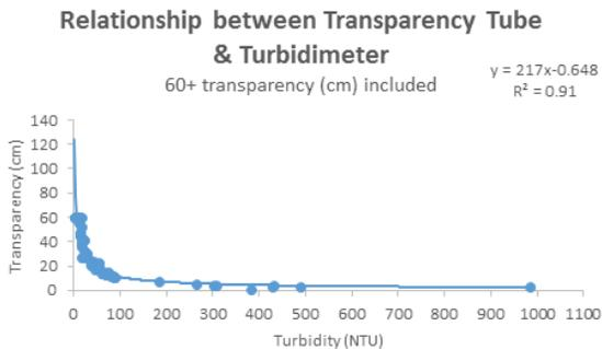
Figure 43 – Relationship between the lab transparency and turbidity measurements
