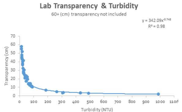
Figure 44 – Relationship between lab transparency and turbidity measurements
