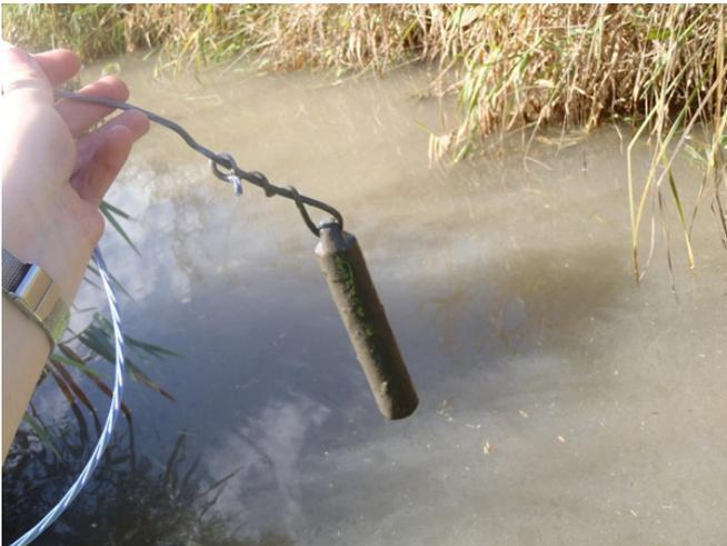
Figure 12 – Pressure transducers buried in mud at the Ankeny sampling site
