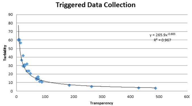
Fig. 50: Correlation of triggered data for transparency and turbidity - all samples
