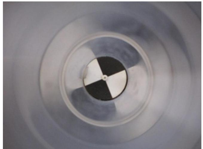
Figure 37 – Image at the bottom of transparency tube
