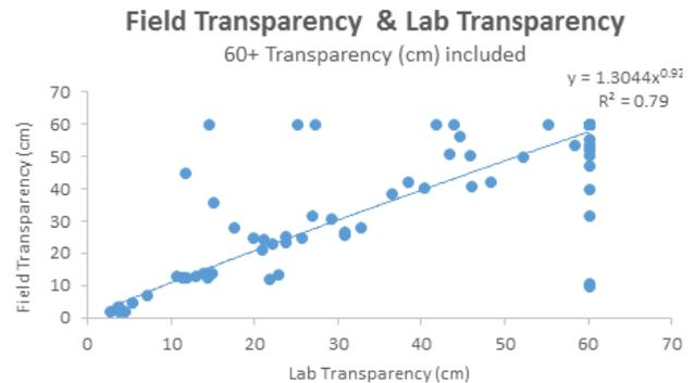
Figure 45 – Relationship between the lab transparency and turbidity measurements
