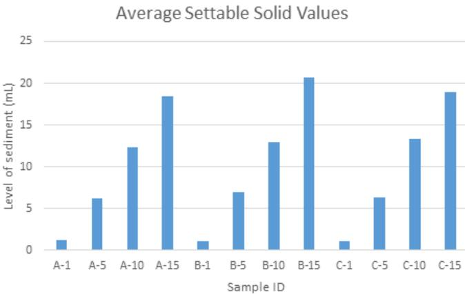
Figure 58 – Average settable solid Values for each soil horizon
