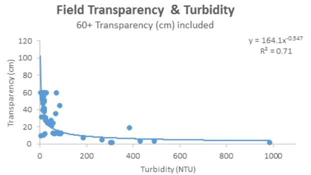
Figure 47 – Relationship between the lab transparency and turbidity measurements
