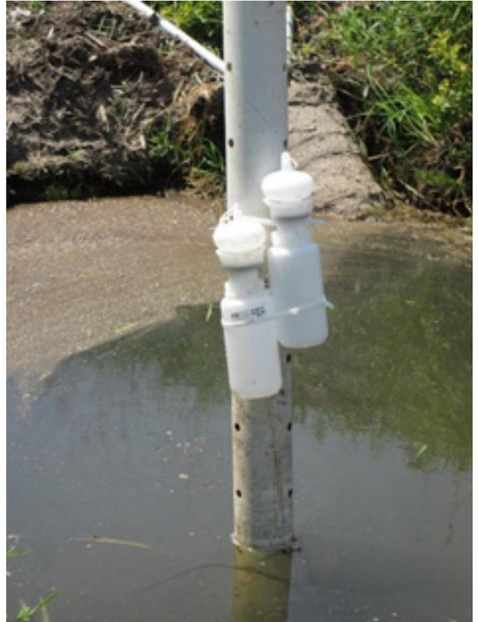
Figure 41- Rising stage sample bottles at AnkUp were set at the given water level at the time of the site visit. After one week with no rainfall, the stream stage dropped dramatically.
