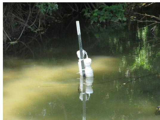
Figure 3 – Assembled rising stage sampler
