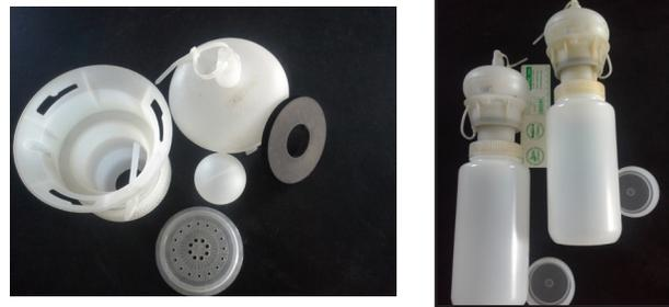
Figure 2 – Rising stage sampler bottle
