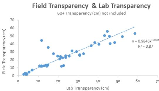
Figure 46 – Relationship between the lab transparency and turbidity measurements
