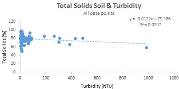
Figure 57 – Relationship between total solids soil and field turbidity measurements.
