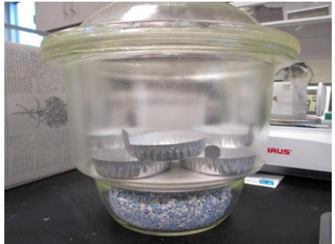
Figure 39 – Desiccator containing Total Solids soil samples
