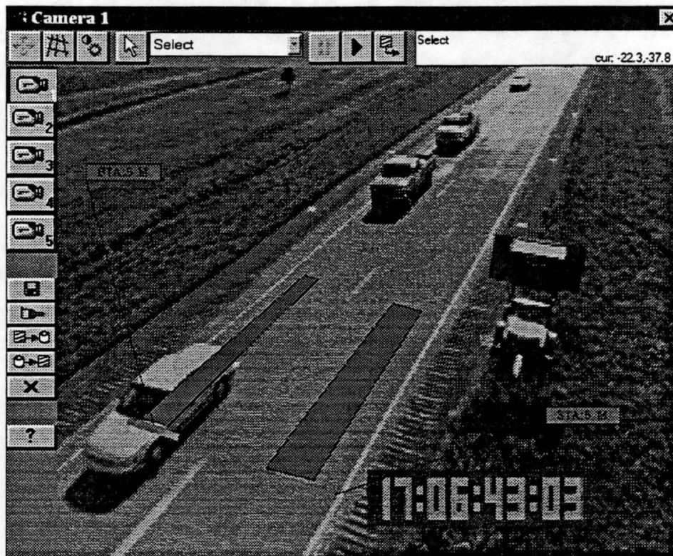
Figure 5-2 Example of Virtual Detectors Placed over Video Image
