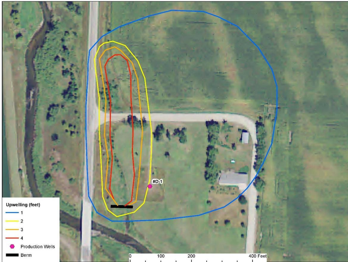
**Figure 19.** Proposed earthen berm location and simulated upwelling near Well D-1.
