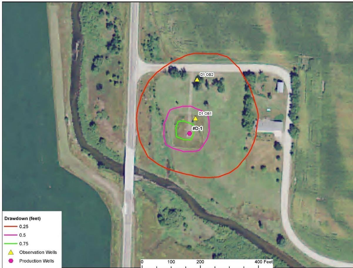
**Figure 12.** Simulated drawdown near well D-1 used in model calibration in Table 10.
