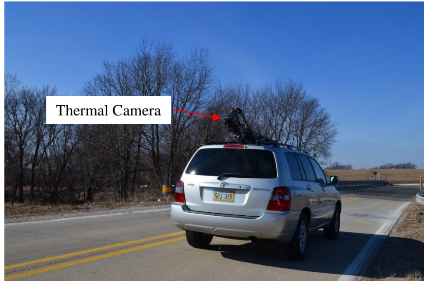
Figure 3.13. Thermal image scanning of Mud Creek Bridge using thermal camera mounted on a vehicle
