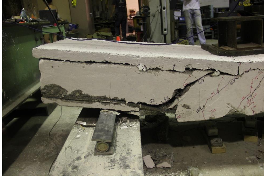
Figure 4.17. Damage to UHPC-NC interface after specimen reached peak load and shear failure ensued
