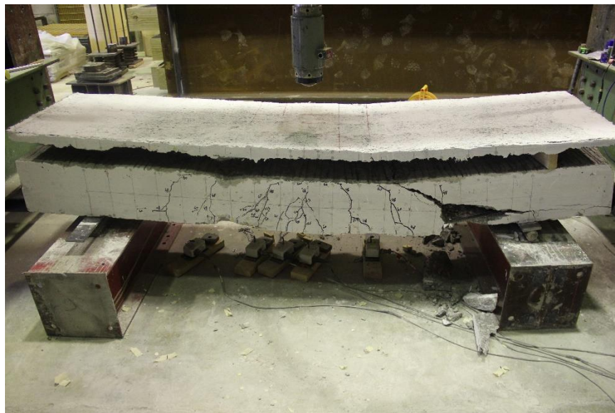
Figure 4.18. UHPC layer pried open after the test
