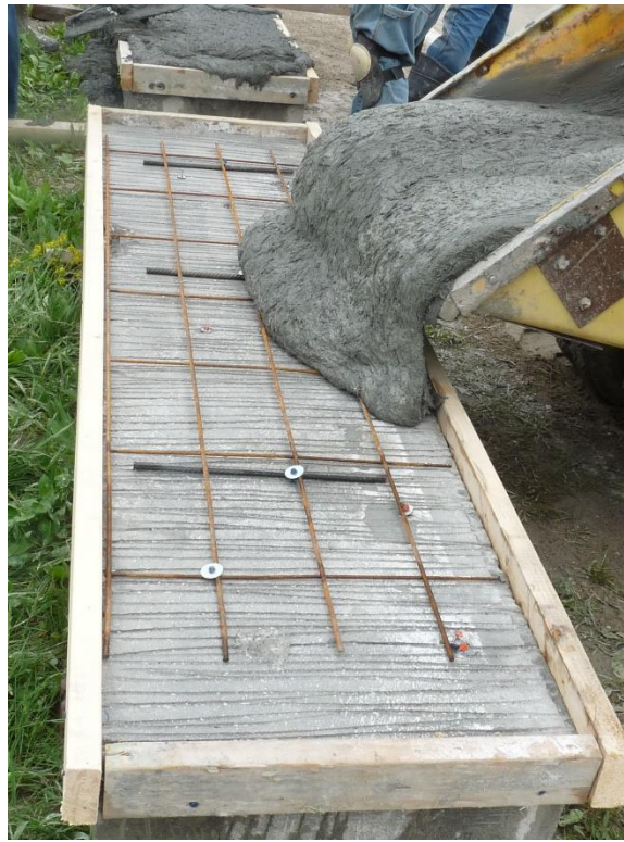
Figure 4.2. Pouring of UHPC overlay on the slab specimens
