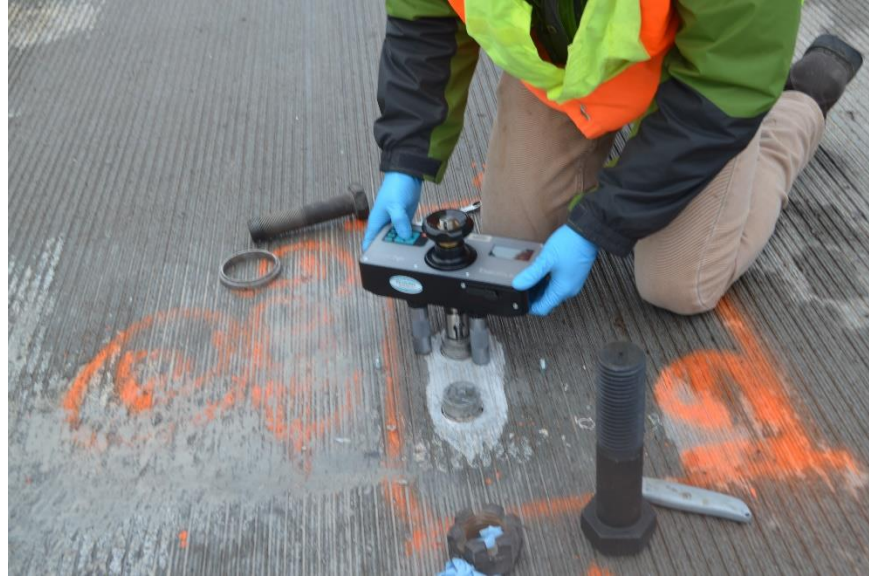
Figure 3.11. Pull-off test on Mud Creek Bridge deck
