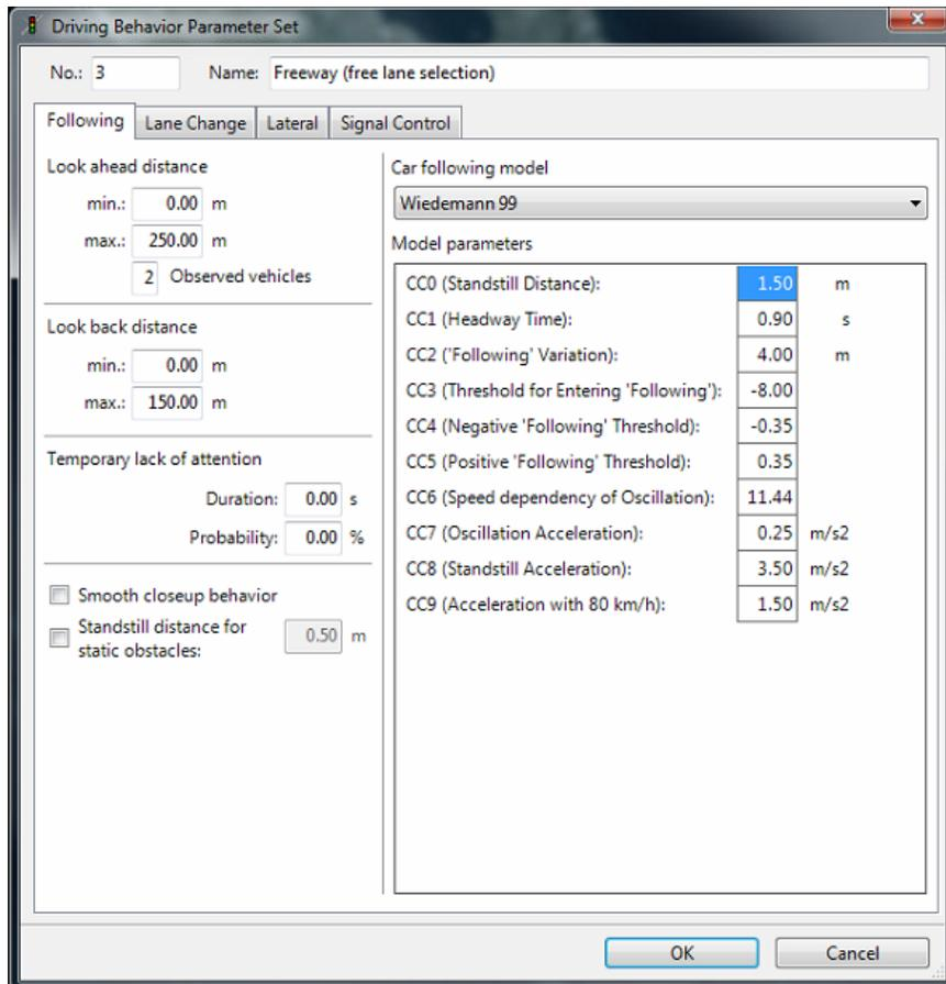
**Figure 5.2. VISSIM car following parameters**
