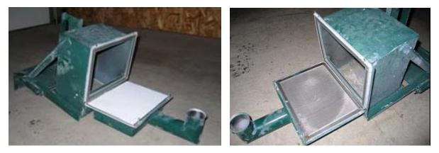
Figure 5.1.5. Opened filter box with and without filter paper.
