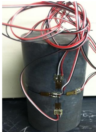
Figure 3.6. Strain gauges on specimen
