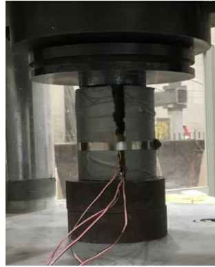
Figure 3.5. Compressive strength test setup
