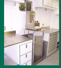
AVA setup procedure in the PCC Center Mobile Concrete Research Lab: convert counter, remove floor portal door, lower weather shield through the floor portal, place three-legged stand on the ground protected by weather shield, place deck on top of stand, place AVA on top of deck.
