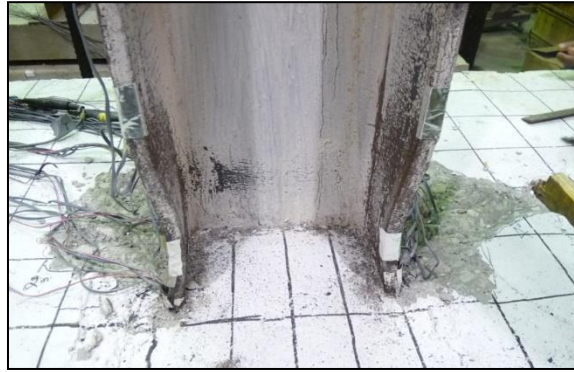
Figure 5-20. Buckling of HP 10 × 57 steel pile and spalling at top surface of abutment cap
