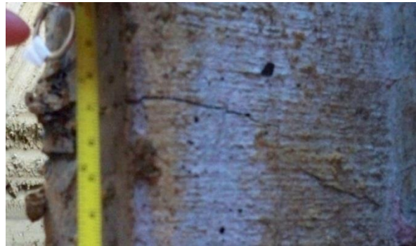
Figure 6-54. Flexural crack found 9 ft from the ground surface on P4 due to the lateral load test
