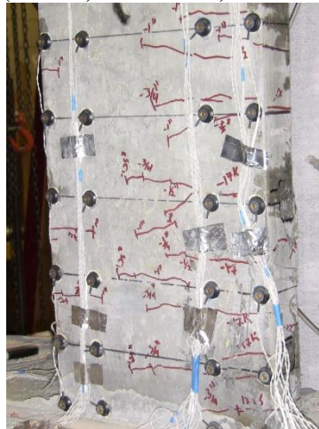
d) Cracking in pile flange at 1.25 in. top displacement (Phase III)
