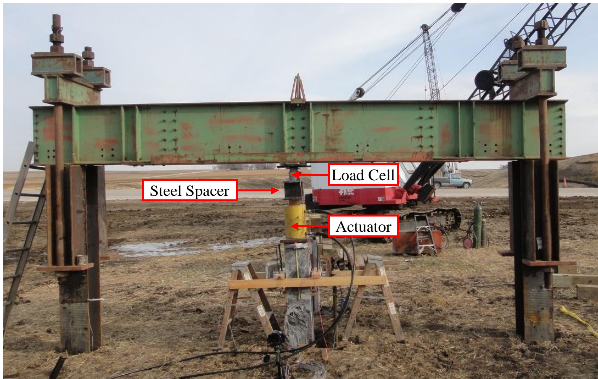
Figure 6-31. Completed axial load test setup
