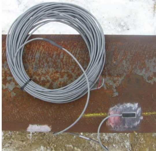
Figure 7-4. Weldable steel strain gages used to monitor steel HP 10 × 57 production piles
