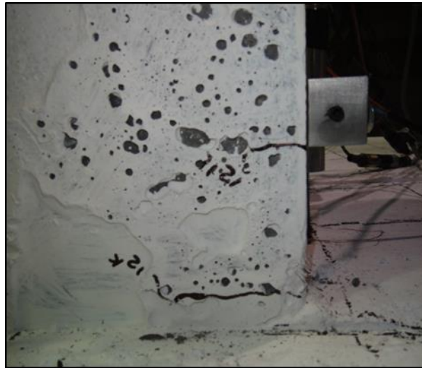
Figure 5-24. Hairline tensile cracks on UHPC pile in UPAC-1 at 12 kip lateral load step with 100 kip axial load
