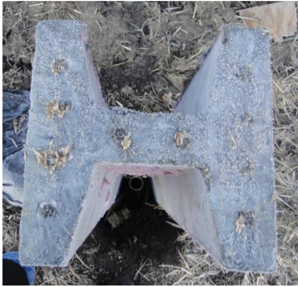
Figure 6-27. No visible damage on P4 pile head after driving
