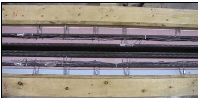
Figure 5-5. Threaded \frac{1}{4} in. coupler inserts in the UHPC pile formwork to attach instrumentation
