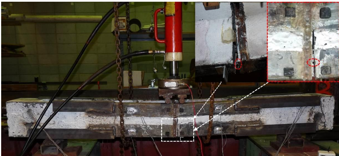
Figure 4-17. Failure of test specimen in weak-axis bending and close-up of the failed welds
