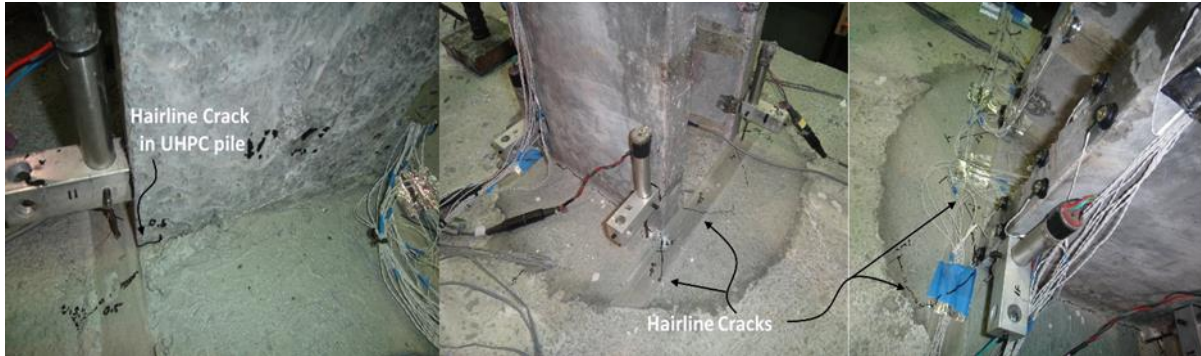
(a) Cracking at 0.5 in. lateral displacement during Phase III testing
