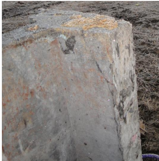
Figure 6-26. Slight damage observed to P3 pile head after driving the pile in place
