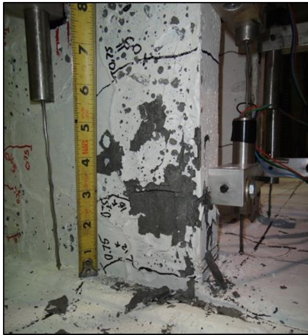
Figure 5-25. Spalled region of the UHPC pile due to crushing during the UPAC-1 test after completing of the 1.0 in. load displacement cycles
