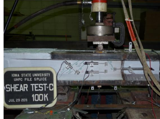
b) Shear cracking in web region of pile
