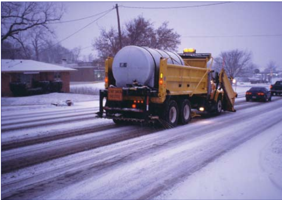
Figure 7–8. Urban application of deicing chemicals (WDM)
