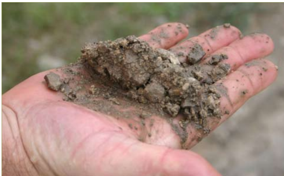
Figure 3–4. Moisture test: wet
