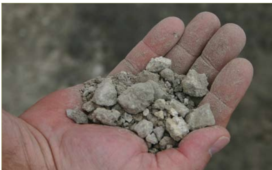
Figure 3–5. Moisture test: too dry
