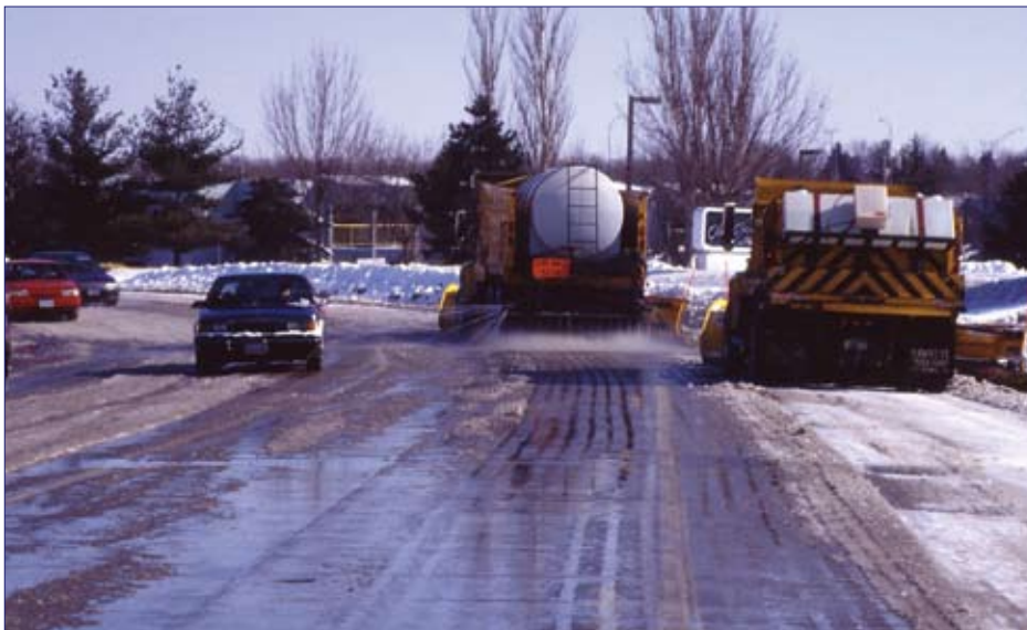
Figure 7-2. Urban anti-icing operations (WDM)
