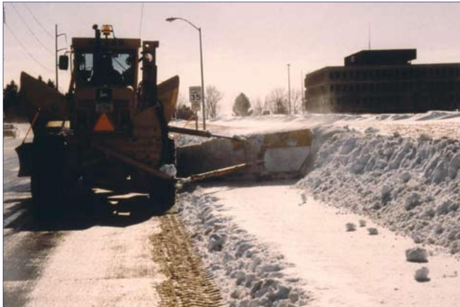
Figure 7-6. Winging operations (WDM)
