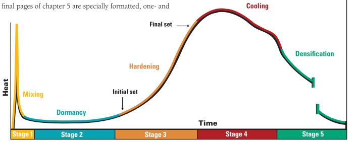
Figure 3. The five stages of hydration mapped on a heat vs. time curve
