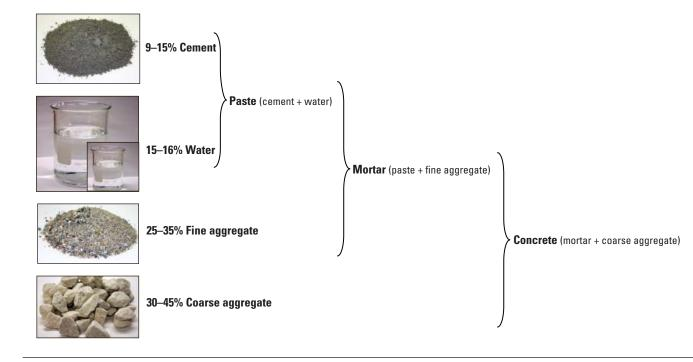
Figure 1. Concrete is basically a mixture of cement, water/air, and aggregates (percentages are by volume).
