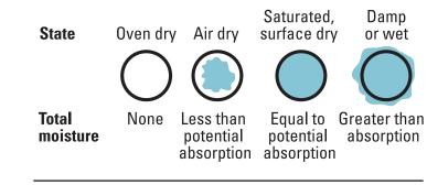
Figure 2. Saturated, surface dry (SSD) is typically the preferable aggregate moisture state.
