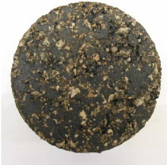
(a) Gyratory compacted specimens (40°C)
