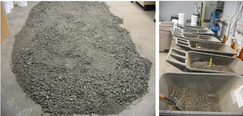
Figure 5-1. Drying process of the RAP materials at the laboratory
