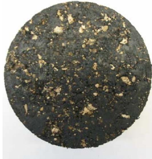
(b) Gyratory compacted specimens (60°C)
