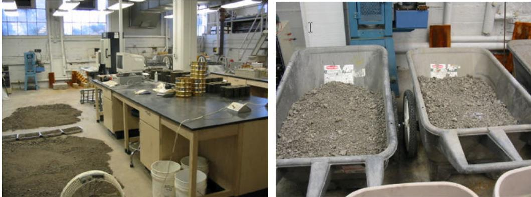
Figure 10-23. Drying process of the RAP materials at the laboratory
