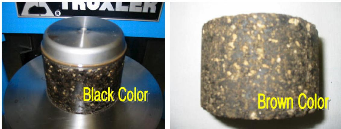
(a) Gyratory compacted specimens (50 G) (b) Marshall compacted specimens (75 blows)
