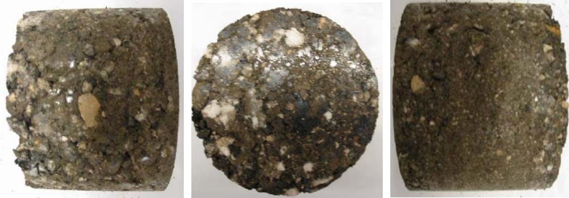
(a) RAP specimens without foamed asphalt and water
