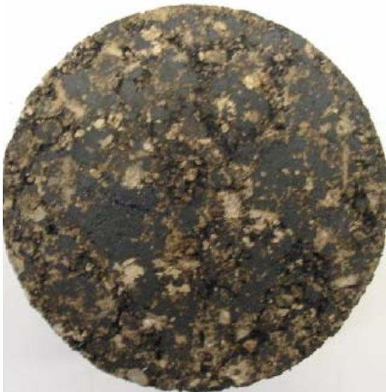
(c) Marshall compacted specimens (40°C)
