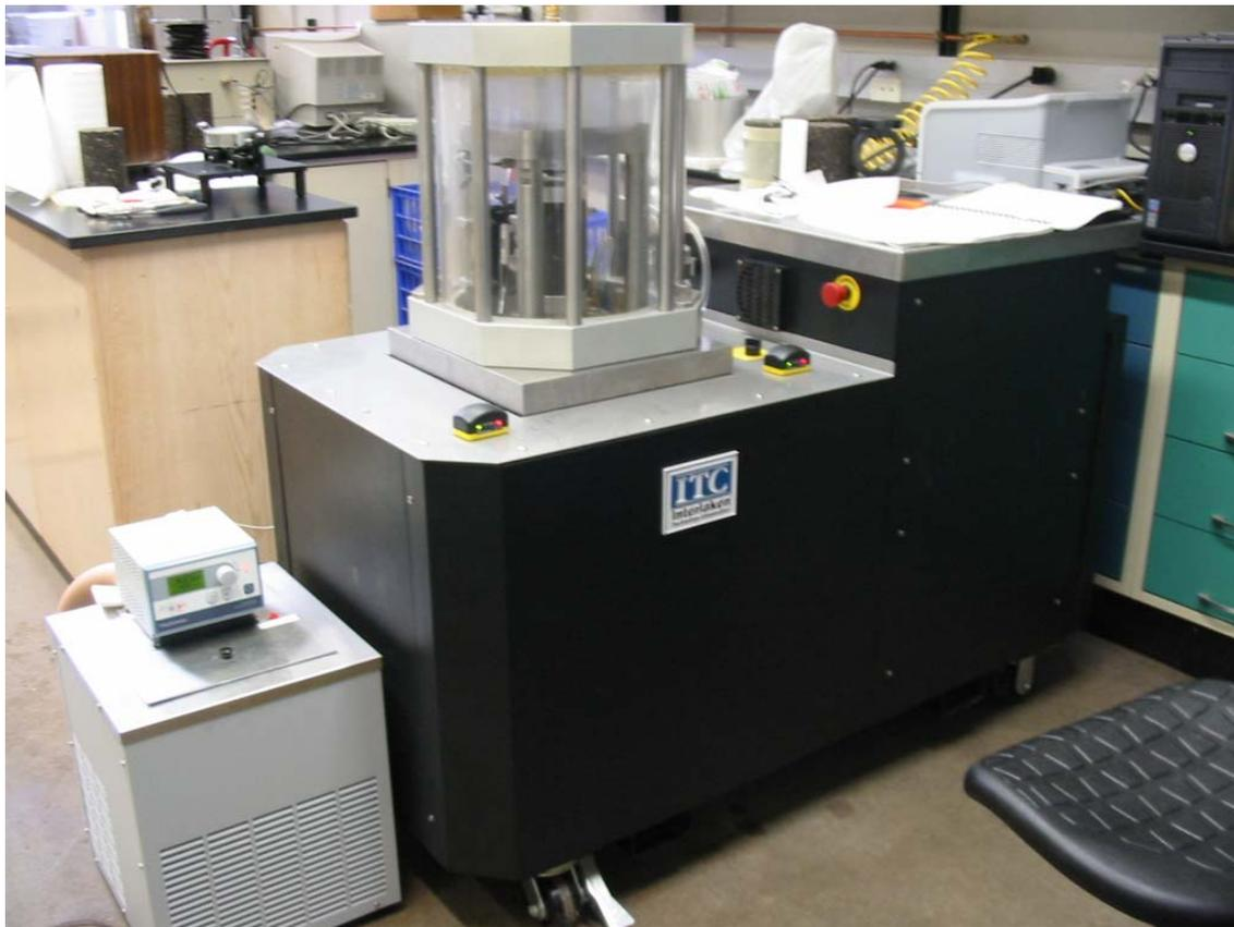
Figure 8-2. Simple performance testing equipment
