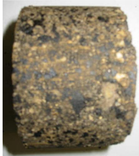
(b) Marshall compacted specimens
