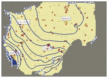
**Figure 3.** Visual MODFLOW results showing the regional groundwater contours (potentiometric surface). Red symbols = production wells and contours are in meters.
