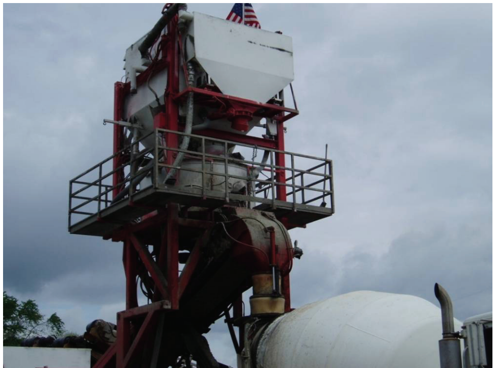
A two stage PCC mixing tower
